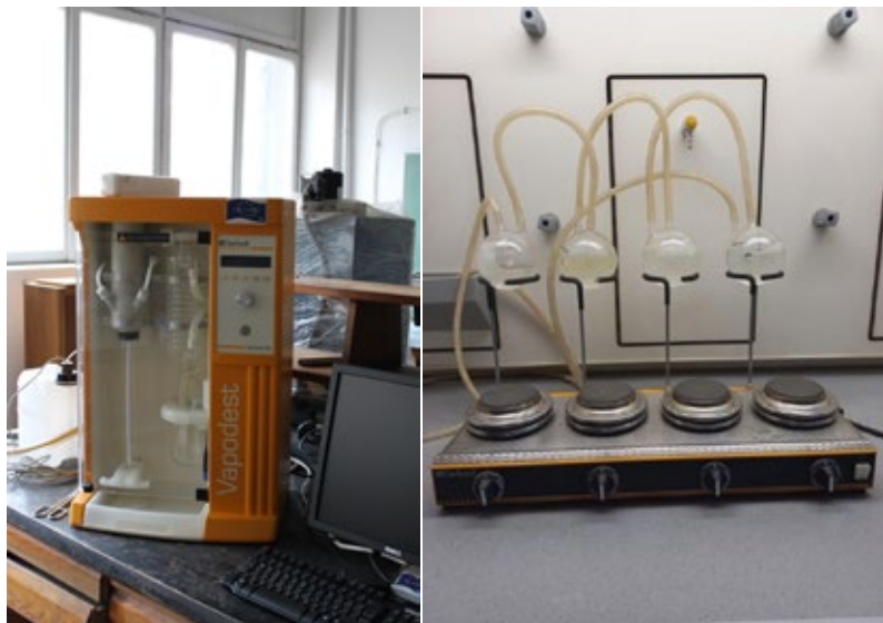
Kjeldahl – for determination of nitrogen and proteins and Soxterm– for hydroanalysis
